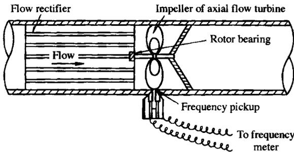
Fig. 11.12 Turbine flowmeter
