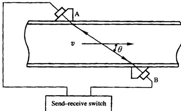
Fig. 11.14 Ultrasonic flowmeter
